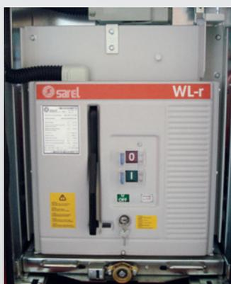
The MV vacuum circuit breaker WL/r encapsulated type is fully withdrawable, the CB can only be racked out of the switchgear only when the door is closed, for the maximum safety. Thanks to a special production process, it ensures high performances under all service conditions.
